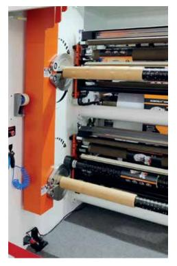
converting unit for flexible packaging. To fully appreciate this statement, you only need to consider the fact that unlike most other machines, slitter rewinders are required to slit and rewind multiple coils, with each coil conforming to the quality norms of the customer.
