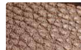
3D leather structure with a depth of 300 µm
